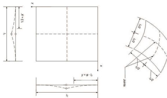
Figure 3.1: The design model of composite shell with longitudinal and transversal hinges.
