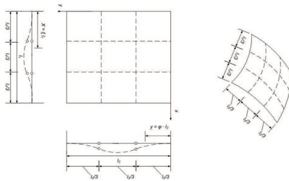
Figure 3.3: The design model of composite shell with two longitudinal and two transversal hinges.
