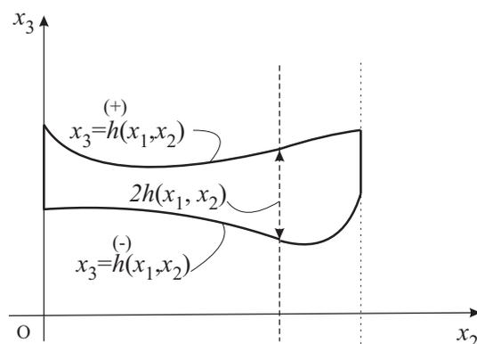
Fig.1. A cross-section of a typical non-cusped prismatic shell
