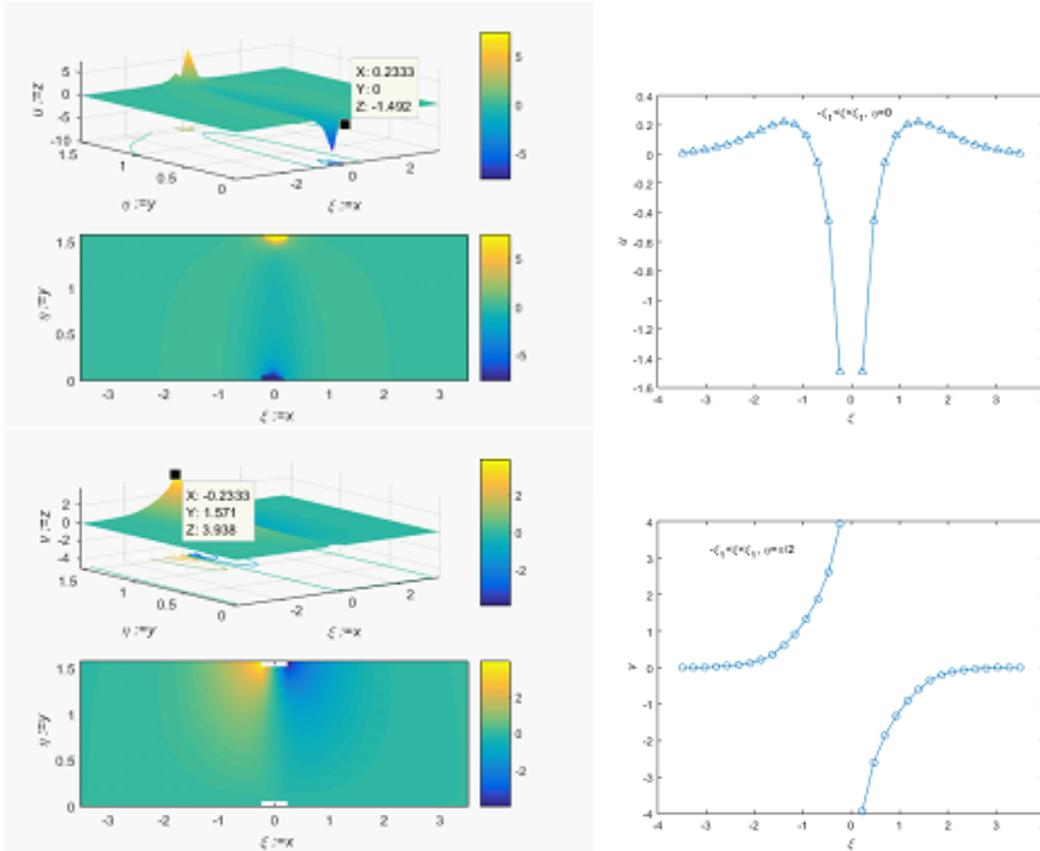
Figure 3. Distribution of displacements in the area bounded by lines  $\eta = 0$ ,  $\eta = \eta_1$  and  $\xi = \pm\xi_1$  when conditions (10a) are valid (normal stress is applied to  $\eta = \eta_1$ . See Fig. 1).
