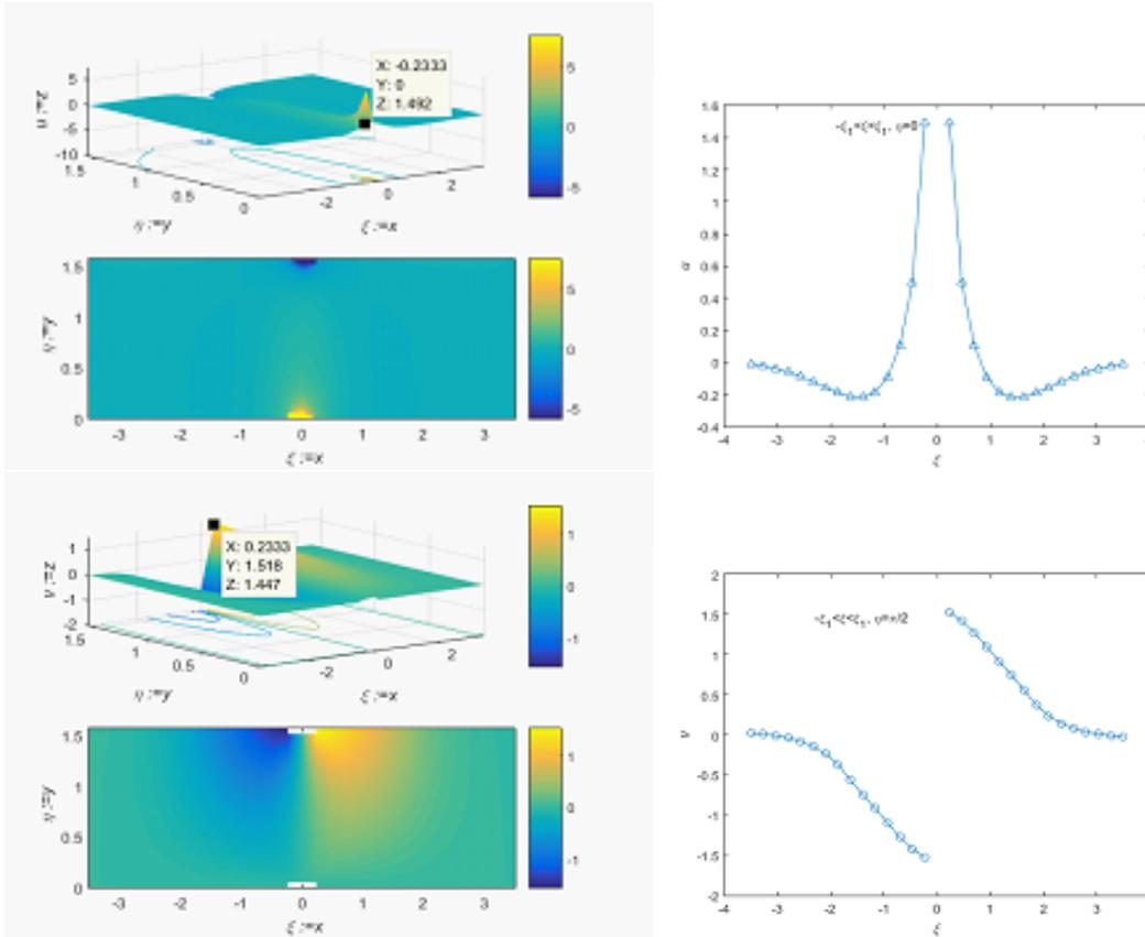
Figure 5. Distribution of displacements in the area bounded by lines  $\eta = 0$ ,  $\eta = \eta_1$  and  $\xi = \pm\xi_1$ , when condition (10a) is valid (tangential stress is applied to  $\eta = \eta_1$ . See Fig. 1).
