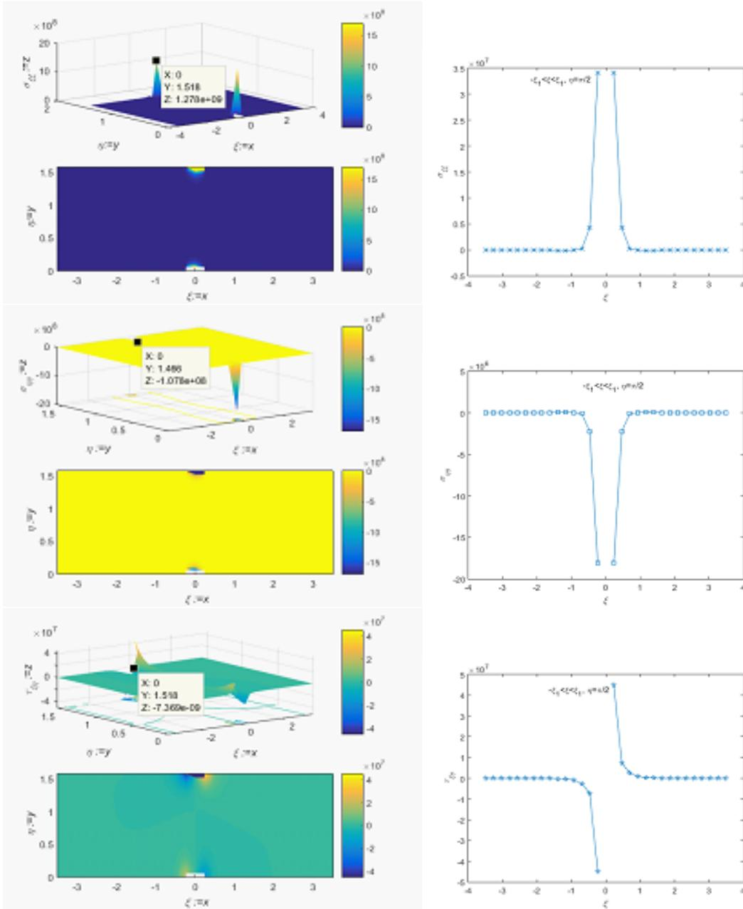
Figure 8. Distribution of stresses in the area bounded by lines  $\eta = 0$ ,  $\eta = \eta_1$  and  $\xi = \pm\xi_1$ , when conditions (10b) are valid (tangential stress is applied to  $\eta = \eta_1$ . See Fig. 1).
