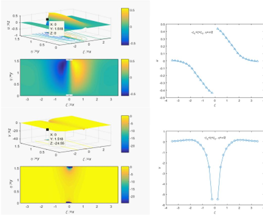
Figure 7. Distribution of displacements in the area bounded by lines  $\eta = 0$ ,  $\eta = \eta_1$  and  $\xi = \pm\xi_1$ , when conditions (10b) are valid (normal stress is applied to  $\eta = \eta_1$ . See Fig. 1).
