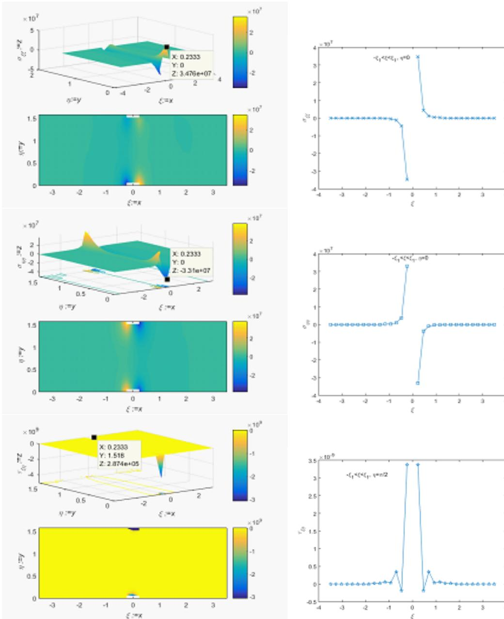
Figure 2. Distribution of stresses in the area bounded by lines  $\eta = 0$ ,  $\eta = \eta_1$  and  $\xi = \pm\xi_1$  when conditions (10a) are valid (normal stress is applied to  $\eta = \eta_1$ . See Fig. 1).
