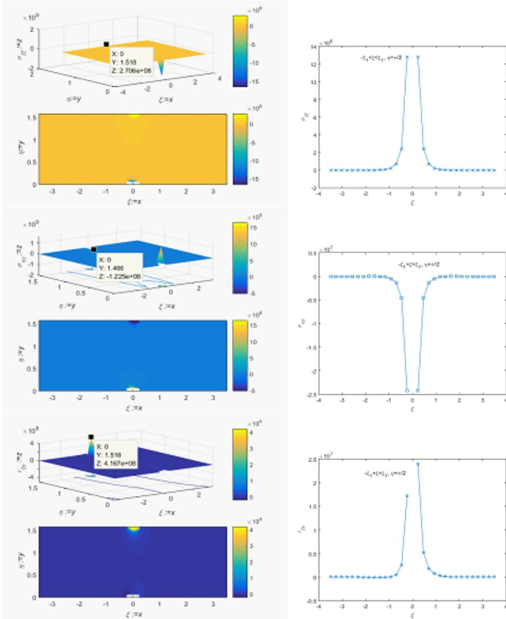
Figure 6. Distribution of stresses in the area bounded by lines  $\eta = 0$ ,  $\eta = \eta_1$  and  $\xi = \pm\xi_1$  when conditions (10b) are valid (normal stress is applied to  $\eta = \eta_1$ . See Fig. 1).
