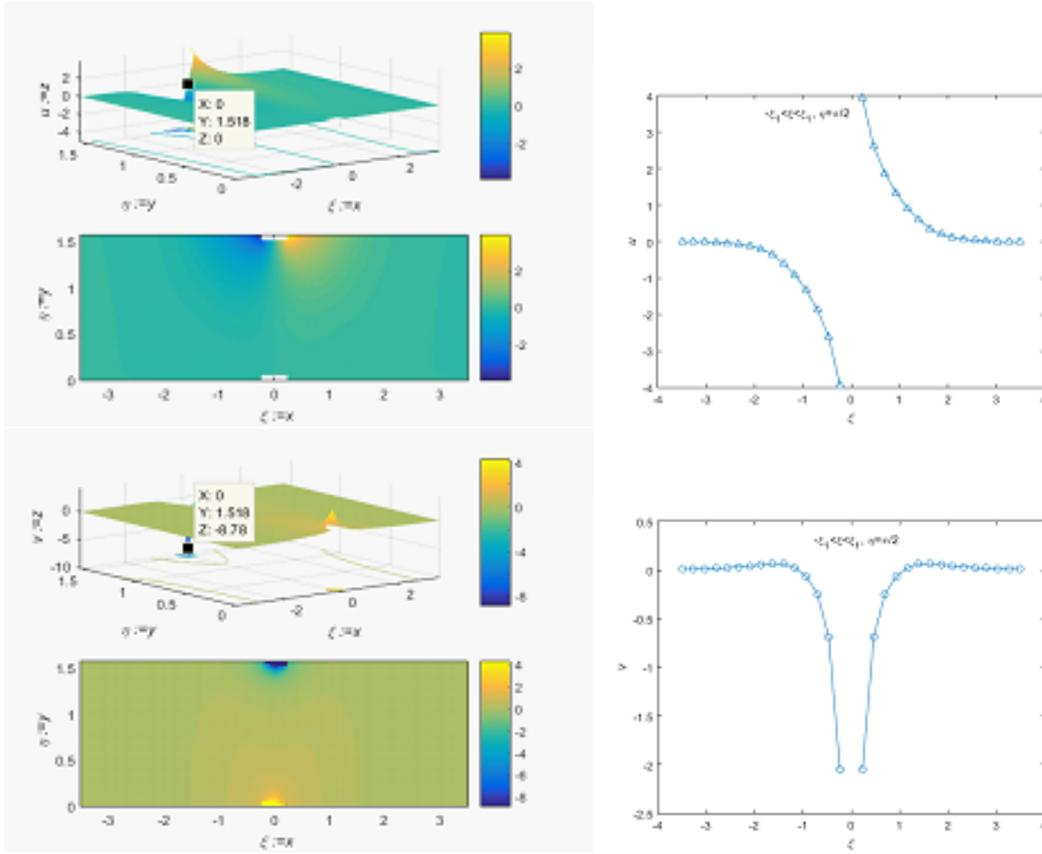
Figure 9. Distribution of displacements in the area bounded by lines  $\eta = 0$ ,  $\eta = \eta_1$  and  $\xi = \pm\xi_1$ , when conditions (10b) are valid (tangential stress is applied to  $\eta = \eta_1$ . See Fig. 1).
