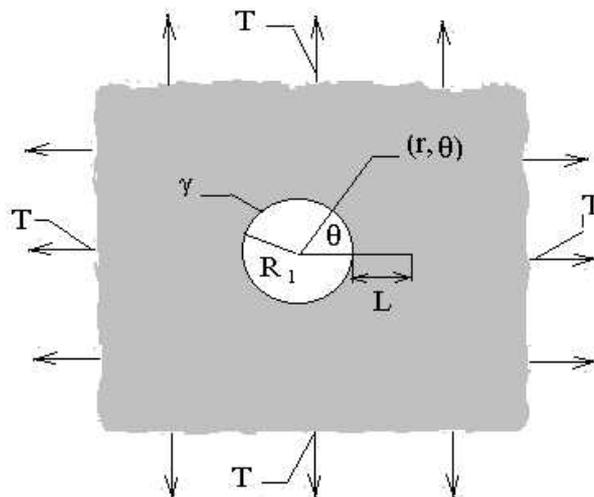
Fig.1. Geometry and loading for the single crack ( $k=1$ ).
