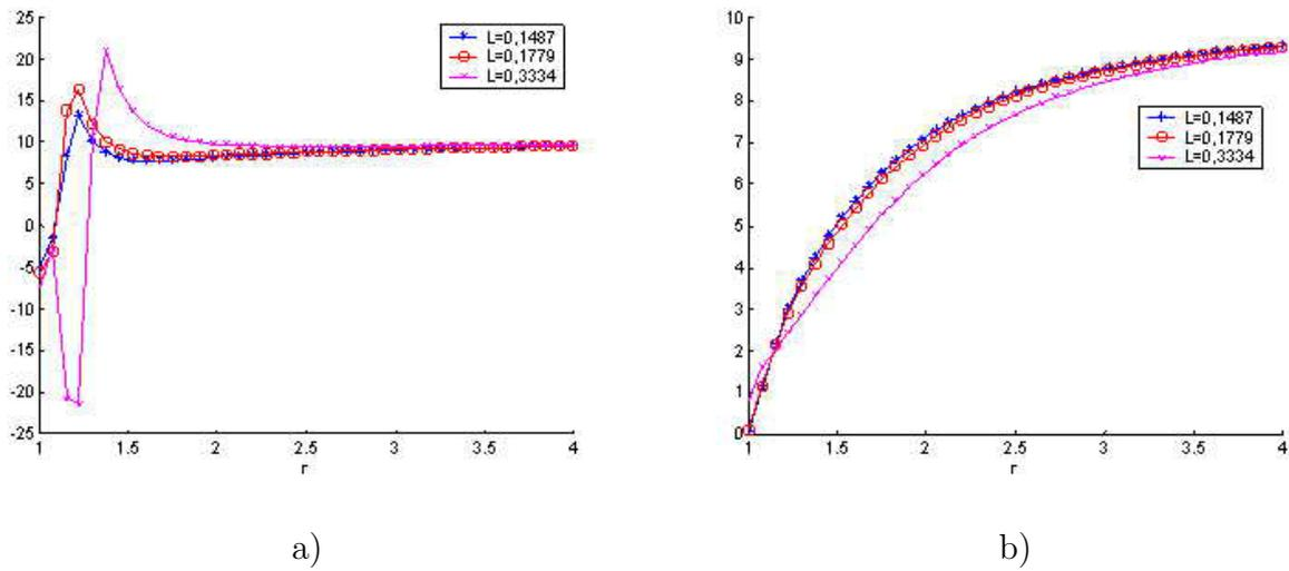
Fig.2. Normal stresses  $\sigma_r$  for  $R_1 < r < 4$  and a)  $\theta = \pi/180$ , b)  $\theta = \pi/4$
